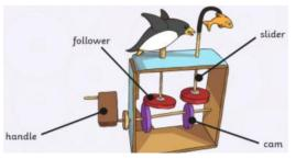
Here are some different examples of cam mechanisms. Each one causes a cam toy to move in a different way.
